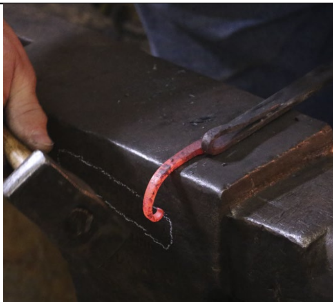
Photo 6: Scrolling the First Tapered Leg
