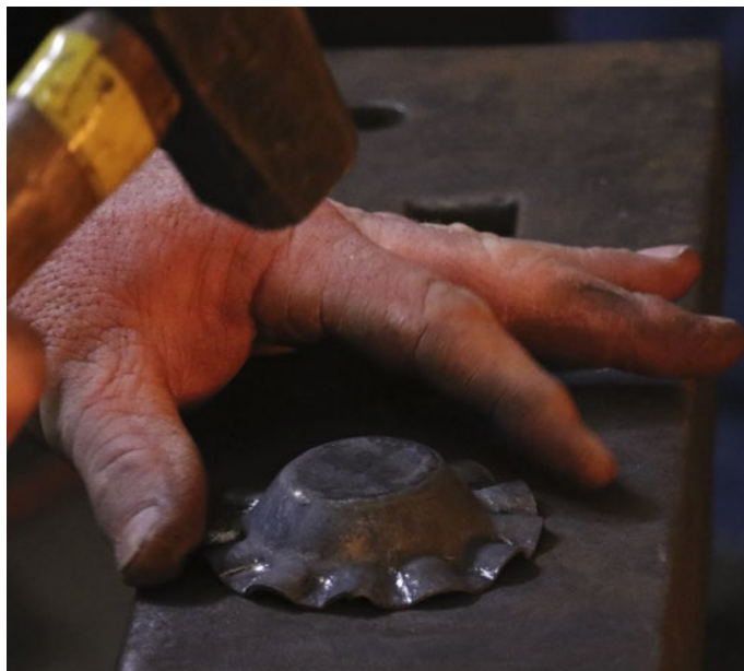
Photo 19: Truing Up the Overall Cup Shape
