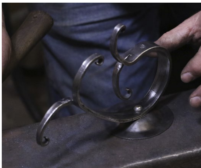
Photo 27: Straightening the Base and Body
