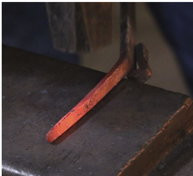
Photo 3: Taper Each End Piece to 3 1/2" Long
