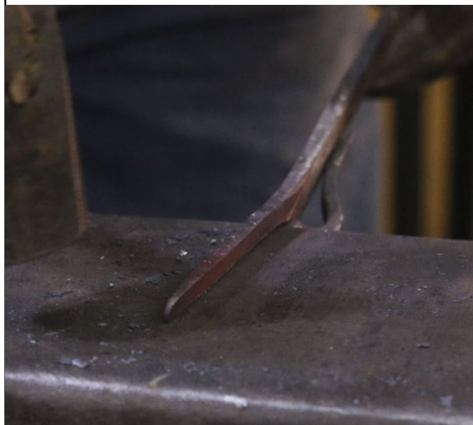
Photo 5: Tapering and Chamfering the Second Leg
