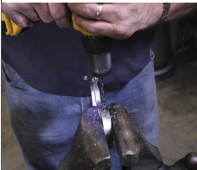
Photo 25: Drilling Rivet Holes in the Body
