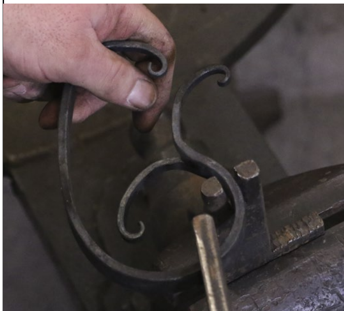
Photo 9: Scrolling the Overall Body Shape
