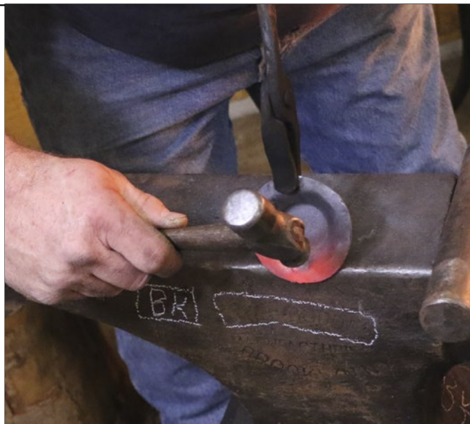
Photo 16: Dressing the Sides on the Anvil Edge
