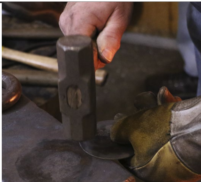
Photo 22: Flattening High Spots on the Base
