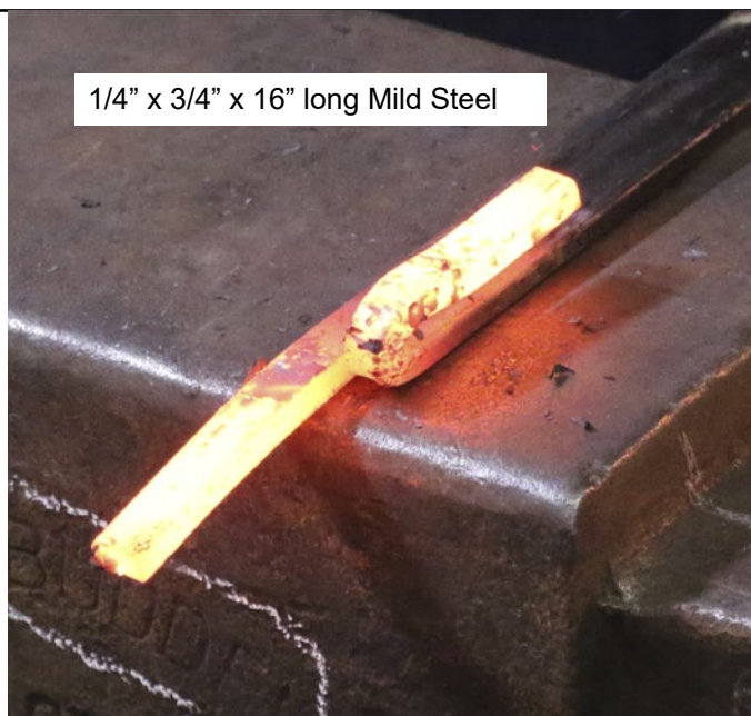
Photo 2: Cut 2 1/2" and Make a Convenience Bend
