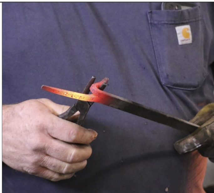
Photo 4: Bending the Unfinished Leg Out for Tapering
