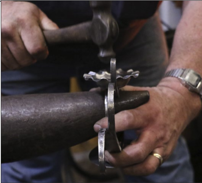
Photo 28: Riveting the Cup to the Body
