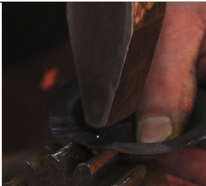
Photo 18: Creating a Wavy Edge on the Cup
