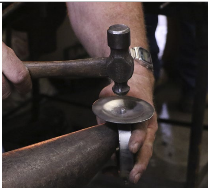
Photo 26: Riveting the Base to the Body
